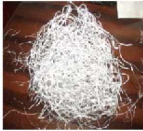
Gambar 7. Bentuk geram continuous chip
